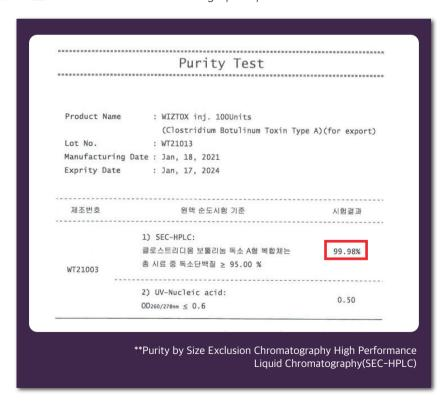
Using Size Exclusion Chromatography High performance liquid chromatography(SEC-HPLC), undiluted toxin complex solution was analyzed which resulted in purity of over 99%.
